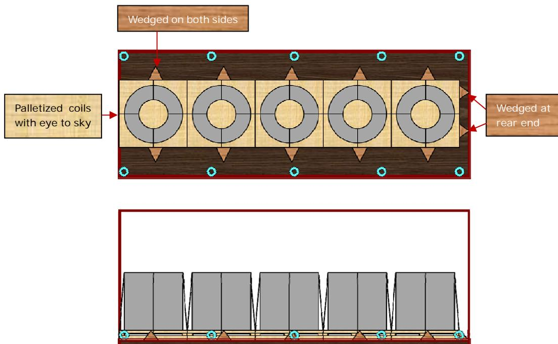
3.3.2. For Coil Weights 5 Tons and up to 7 Tons
